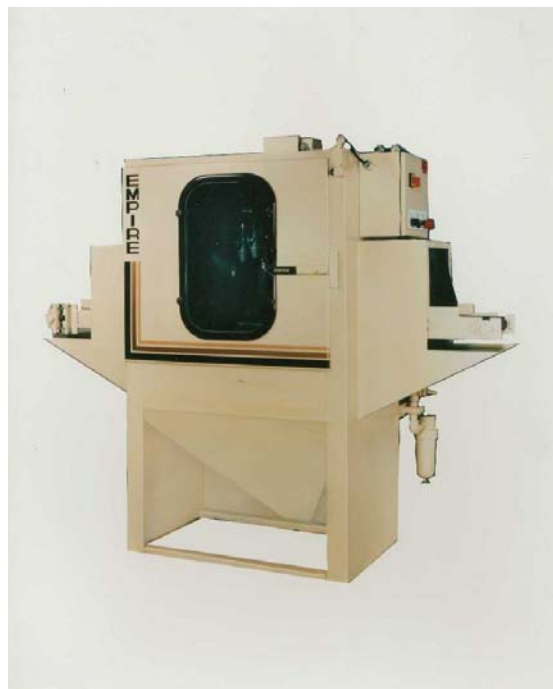
Figure 1 – IL-885 In Line Conveyor System
